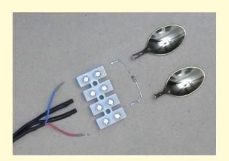
D.1 Screw one espresso spoon and one end of the resistor in one of the outer connectors of the connector strip section. Therefore, first insert the spoon and then place the end of the resistor on the spoon handle stump in the connector. Then screw the second spoon and the other end of the resistor into the other outer pole.
