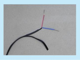
B.7 Thread a **red** heat-shrink tubing over the copper litz wire with the rest of the red insulation.
