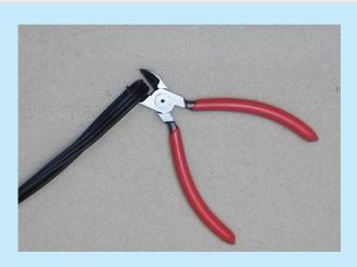
B.1 Cut the 3.5 mm 4-conductor male to male TRRS cable in half. Thereby, you will get two even long cable ends. Only one cable end is going to be used. The second cable end can be kept for a another apparatus.
