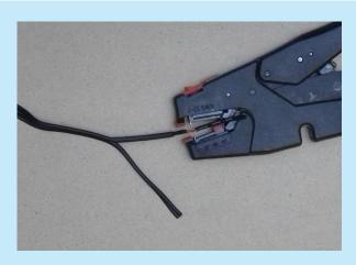
B.4 Remove from the wire with the **red** insulation about 50 mm of the black jacket without damaging the red insulation or the bare copper litz wire.
