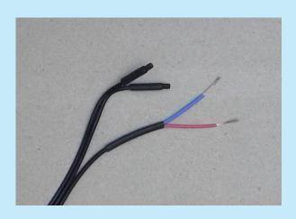
B.9 Put a heat-shrink end cap on each of the unused wires (white and yellow inner insulation).
