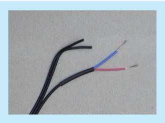
B.8 Pull the **black** heat-shrink tubing a little over the **red** and the **blue** heat-shrink tubing.
