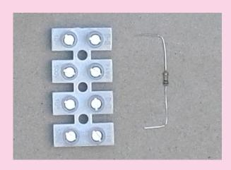
C.1 Bend the ends of the axial-wired resistor so that the straight center is still 40 mm long and the resistor can then be screwed tightly into the outer connectors of the connector strip section.
