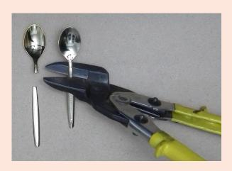
A.1 Cut off the handles of the two spoons with tin snips in a way that the stumps can later be screwed into the screw terminals of the connector strips.
