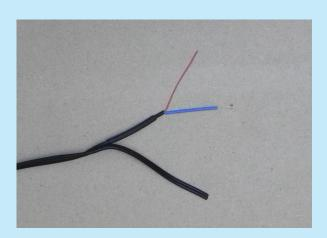
B.5 Thread a **blue** heat-shrink tubing over the bare copper litz wire.
