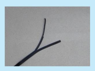
B.3 First, push a black heat-shrink tubing over the cable jacket of the **red** wire until you can see about 70 mm of the wire out of the heat-shrink tubing.
