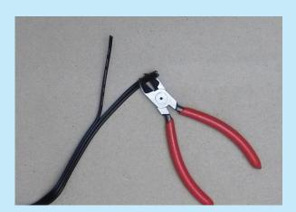
B.2 The **black** ribbon cable consists of three wires. Separate the three wires. In each of the three cable jackets you will find one insulated copper litz wire (**red**, yellow or white) and one non-insulated copper litz wire. For this experiment we only need the wire with the **red** inner insulated wire. Shorten the non-used wires by about 15 mm. We will use them later to build a strain relief.
