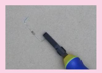
C.2 Crimp the non-insulated wire ferrules onto the ends of the resistor wires.
