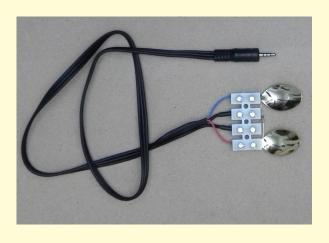
D.2 On the other side of the connector strip section, screw the two wires with the black heat-shrink end caps in the middle connectors. The **red** wire must be connected to the spoon, which will later be held in the left hand. The **blue** wire with the other spoon.
