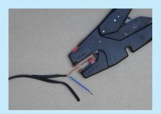
B.6 Use the wire stripper to remove about 30 mm of the **red** insulation.
